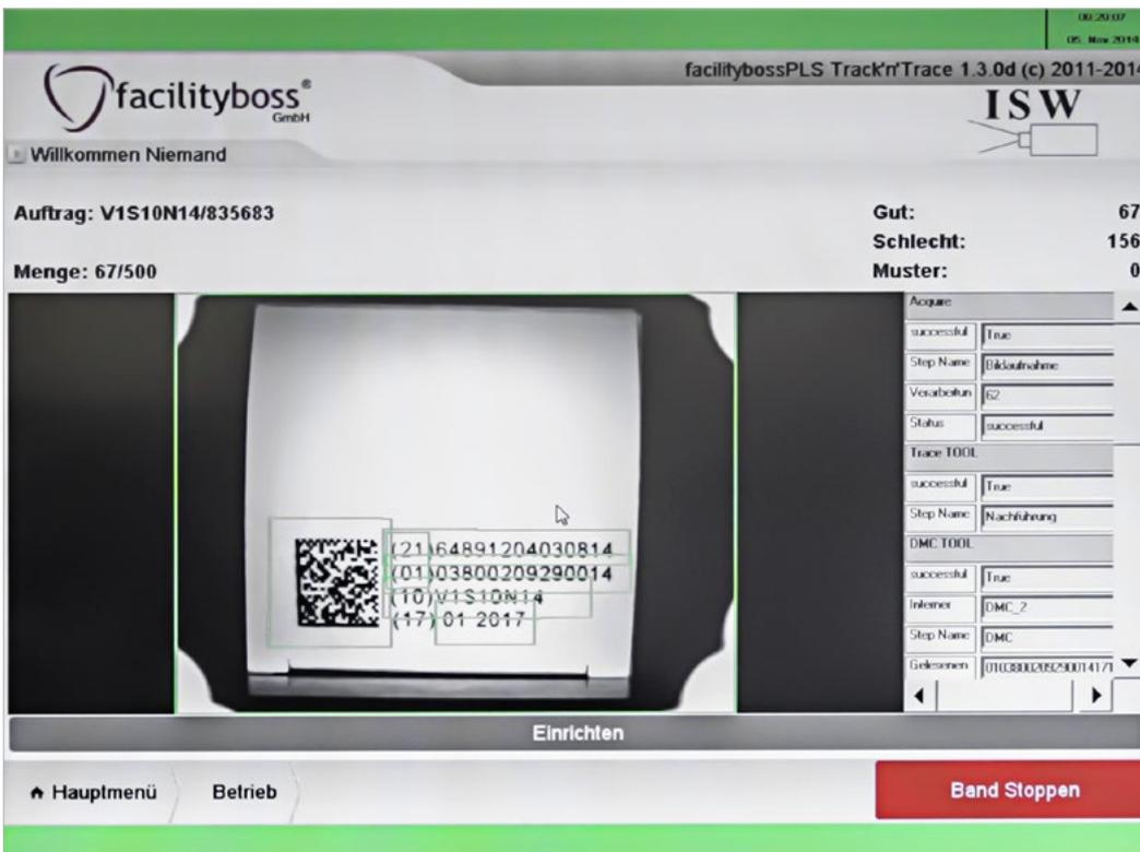
Calibration of the overall system, for example conveyor speed, is via the intuitive HMI which is so easy to operate even in complex parameterization. During operation, the monitor shows at the left the current image together with the respective image processing tool and related parameters at the right.
